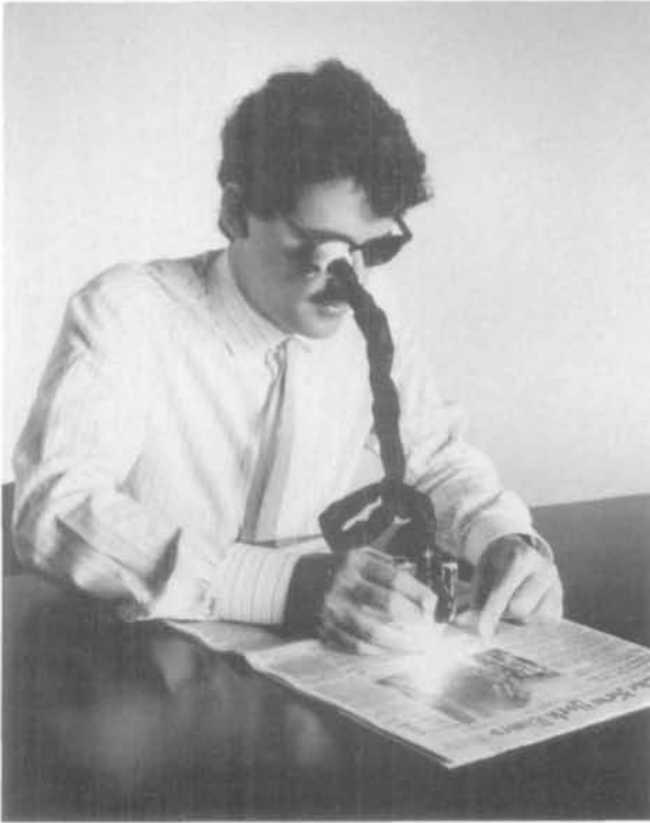
Fig. 3. Fiberscope in use. The eyepiece is supported near the eye, and the user holds the objective in his right hand and slides it over the text. The user is making a V with his left hand to mark the beginning of the line. We have developed several ways of supporting the eyepiece. The eyepiece may be spectacle-mounted as shown here, hand-held, or supported by a stand.
